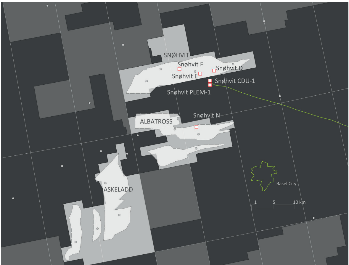
[104] Snøhvit field showing position of production templates (E, D, N), the sub-sea distribution structure (CDU-1) the pipeline end manifold (PLEM-1) and the gas-injection well (F).
