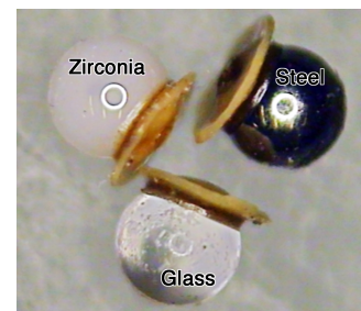
Figure 10. Shorn-off balls, showing rupture mostly between 'cuvette' and 'glue' layer.
