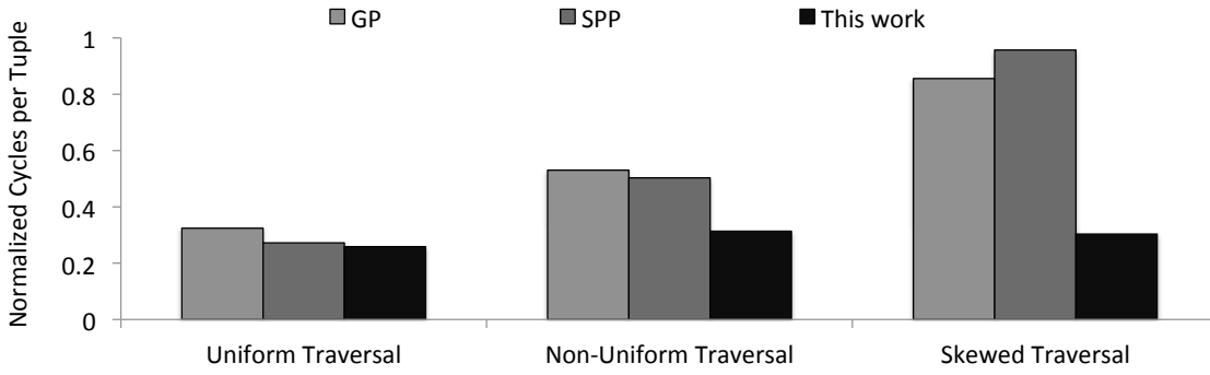
Figure 3.3 – Cycles per lookup tuple normalized to uniform lookups on baseline. Measurement on Xeon x5670.
