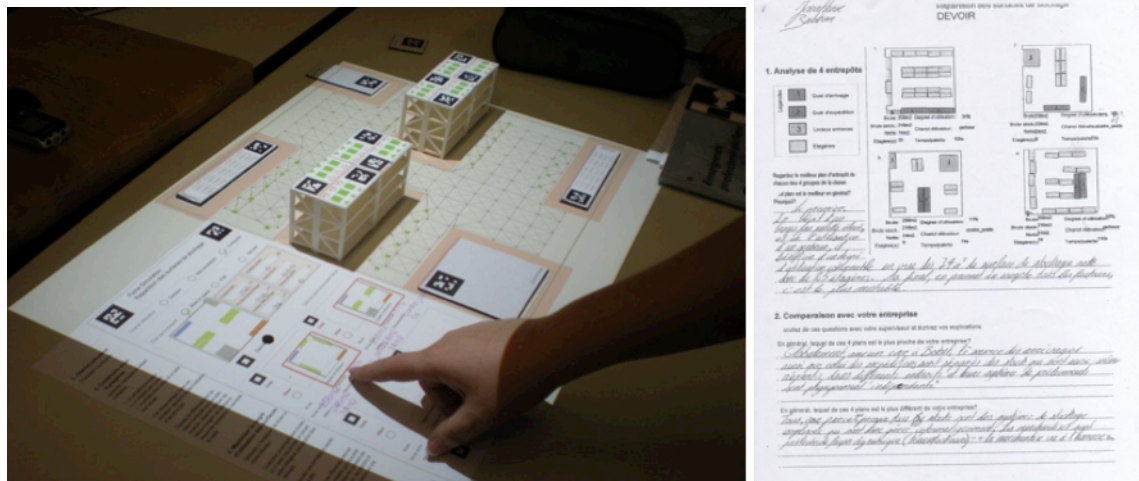
Figure 8. The TinkerLamp activity allowed apprentices simulate the effectiveness of different warehouse layouts (left), fieldwork sheets were used to save their designs to discuss them with their supervisors at the workplace (right).
