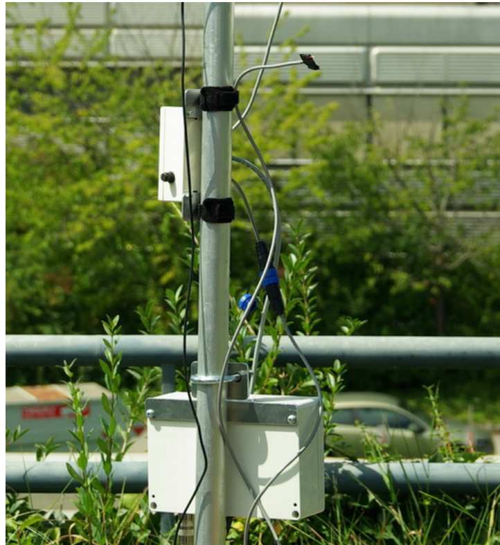
Figure 5.4 – Sensorscope station during outdoor experiment. Modified sensor module (top left) and deployed NTC (top right) are visible.
