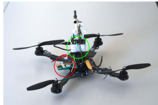
(b) Mounted spectrometer, marked in red. Intermediate sensor board marked in green.
