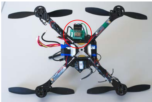
(b) Mounted spectrometer, marked in red. Intermediate sensor board marked in green.
