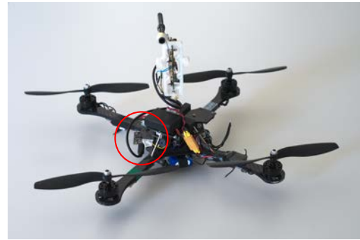
(a) Mounted infrared thermometer, marked in red.
