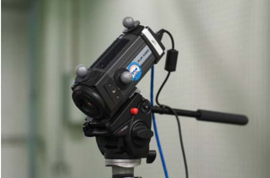
(a) FLIR A320 thermal camera with infrared reflectors for absolute positioning.
