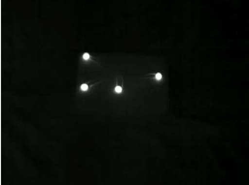
(d) Calibration frame as seen by the thermal camera.
