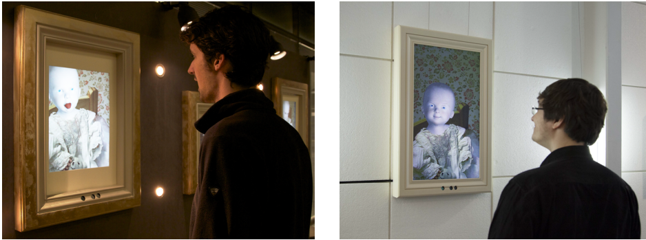
Figure 5.12.: Mimicry , an application case study using our approach. An observer can simply step in front of the picture frame and the character depicted in the virtual painting will start mimicking the person's facial expression in realtime. The sensor is embedded in the frame.
