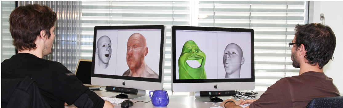
Figure 4.1.: Our system captures and tracks the facial expression dynamics of the users (grey renderings) in realtime and maps them to a digital character (colored renderings) on the opposite screen to enable engaging virtual encounters in cyberspace.
