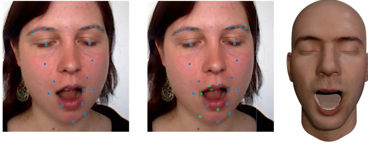
Figure 6.7.: Missing markers can be handled by our retargeting system. The optimization jointly retrieves the location of the missing markers (green) and the target character parameters.
