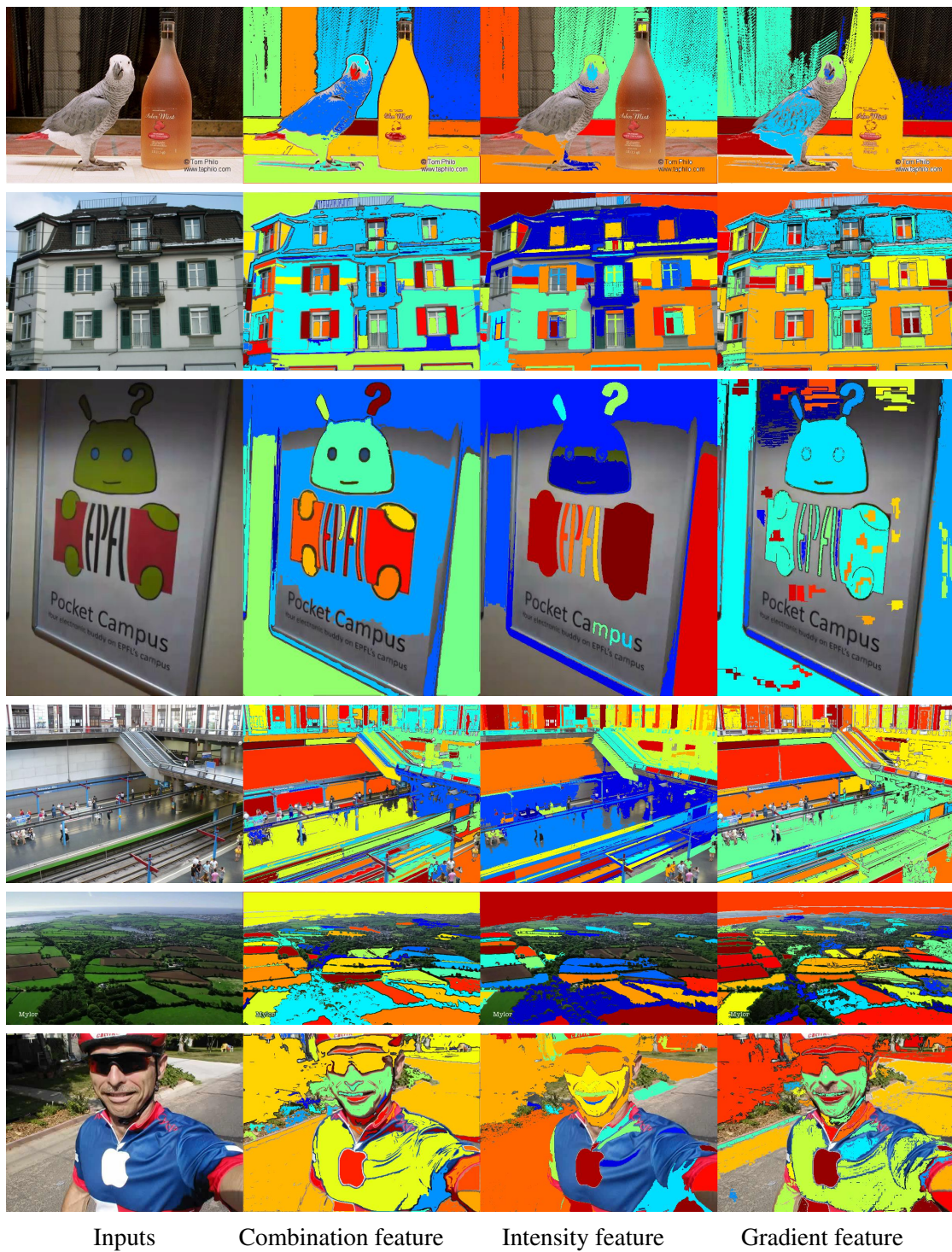
Figure 2.6 – Feature comparison . Component tree segmentation applied to the (middle right) intensity image, (right) gradient image, and (middle left) a combination of intensity and gradient. Detected regions are displayed using a heat map color coding with red indicating highly stable regions and blue low stability. The combination feature works best.
