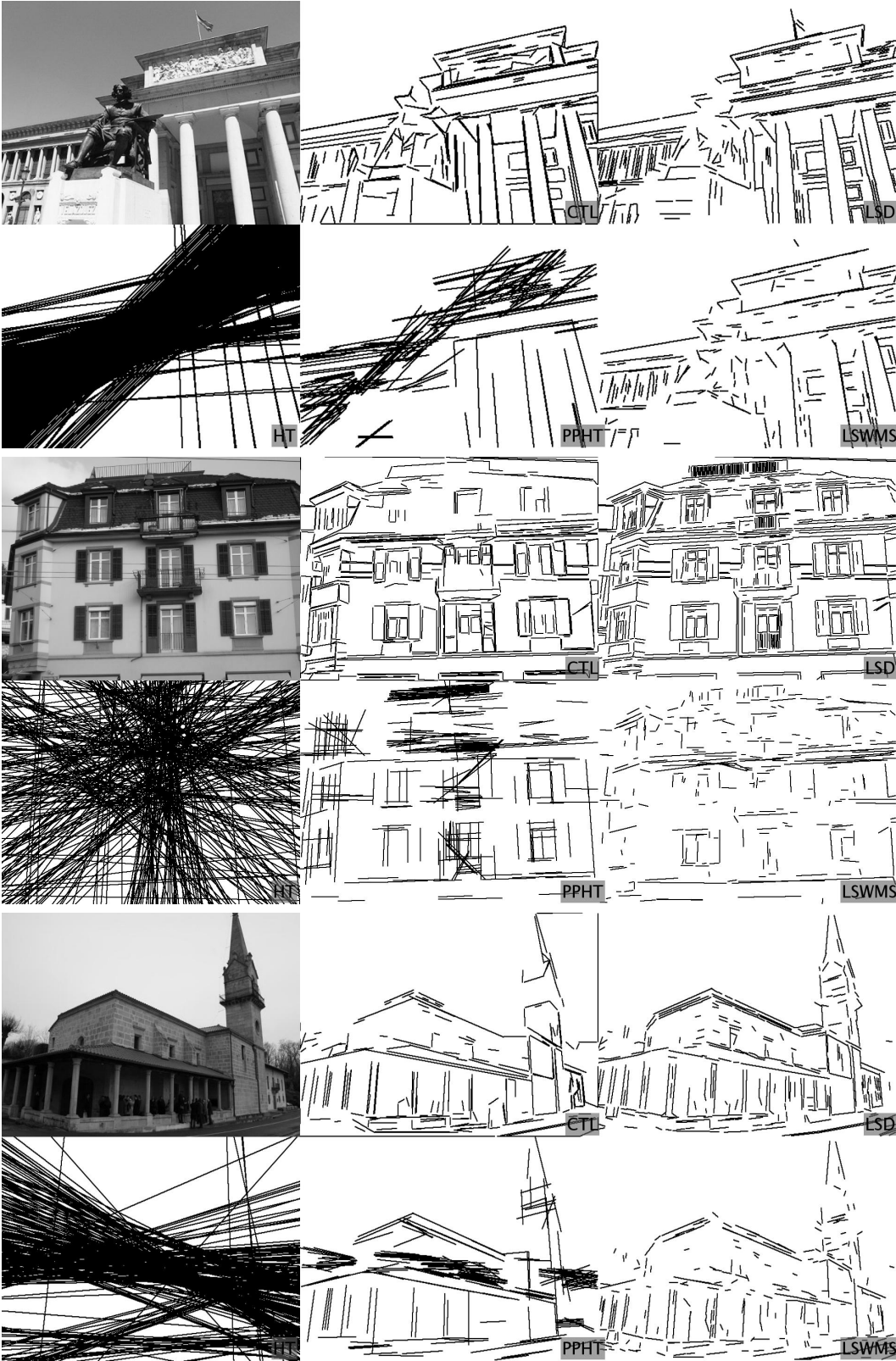
Figure 3.6 – Line segment detection for building facades.
