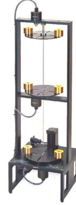
Fig. 3. Torsional apparatus (ECP model 205a) used for the experimental analysis. The three disks are comprised of block masses which can be added or removed to alter the inertia of each disk (and thus alter the dynamics of the system). Each disk is vertically suspended on a spring with a variable spring constant. The actuator is located on the bottom of the device.
