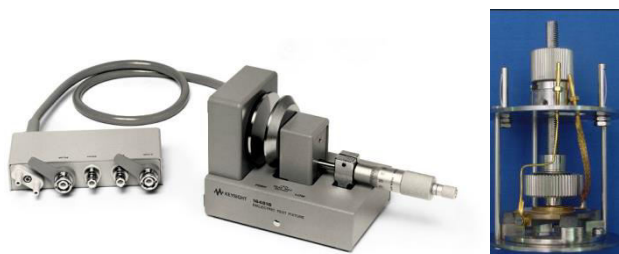
Fig. 71: The setup used for measuring the dielectric properties.
