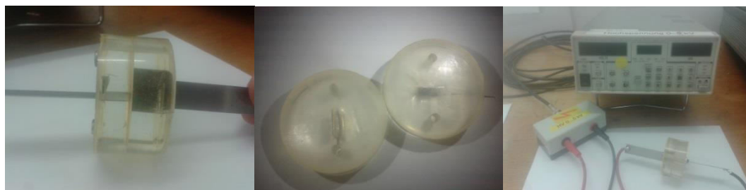
Fig. 70: Electrodes used for breakdown strength measurements and the overall set-up of the system (from left to right).
