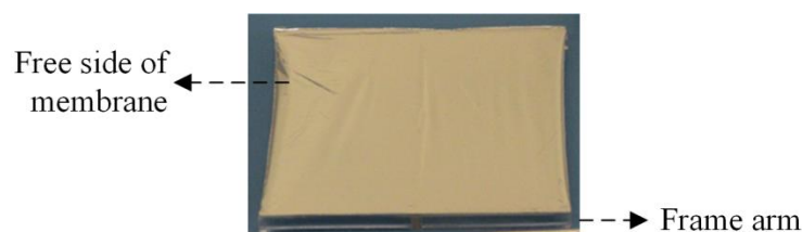
Figure 5.27: Initial experiments on attaching pre-stretched Mylar on a prototype PMMA frame. The free ends of the pre-stretched membrane buckle as shown.
