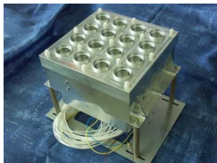
Fig. 1.3: Indium FEEP emitter array from ARCS [29]. 2×2 assemblies as well were extensively tested and characterized. 4 clusters of 9 emitters each (total 36 emitters) were also designed for LISA pathfinder program.
