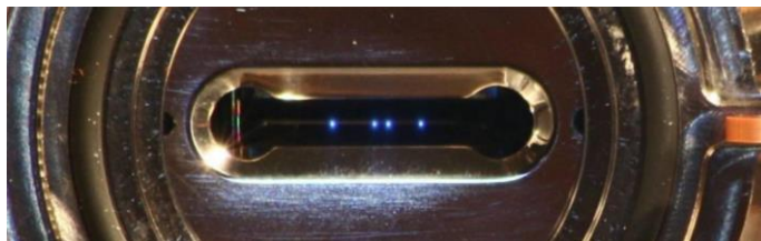
Fig. 1.2: FEEP FT-150 emitter blade at first ignition [31]. Emission starts from few spots on the emitter blade, and it extends progressively to the whole active part of the slit during the initial thrust stabilization phase.
