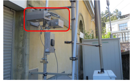
Fig. 1. Two OpenSense II sensor nodes deployed in parallel beside Lausanne NABEL station.
