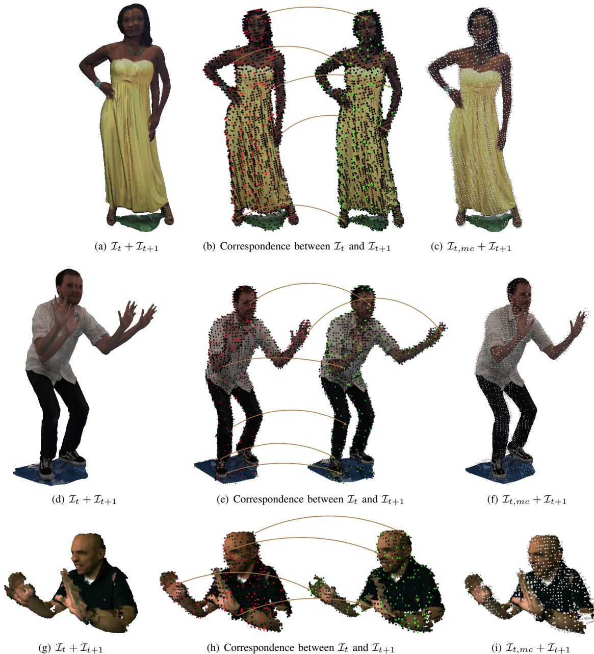
Fig. 9. Example of motion estimation and compensation in the yellow dress, man and upper body motion sequences. The superimposition of the reference ( \mathcal{I}_t ) and target frame ( \mathcal{I}_{t+1} ) is shown in (a), (d), and (g) while in (b), (e), (h) we show the correspondences between the target (red) and the reference frame (green). The superposition of the motion compensated reference frame ( \mathcal{I}_{t,mc} ) and the target frame ( \mathcal{I}_t ) is shown in (c), (f), and (i). Each small cube corresponds to a voxel in the motion compensated frame.
