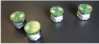
Figure 1: Four Khepera III robots performing one of the learned flocking algorithms presented in this article.
