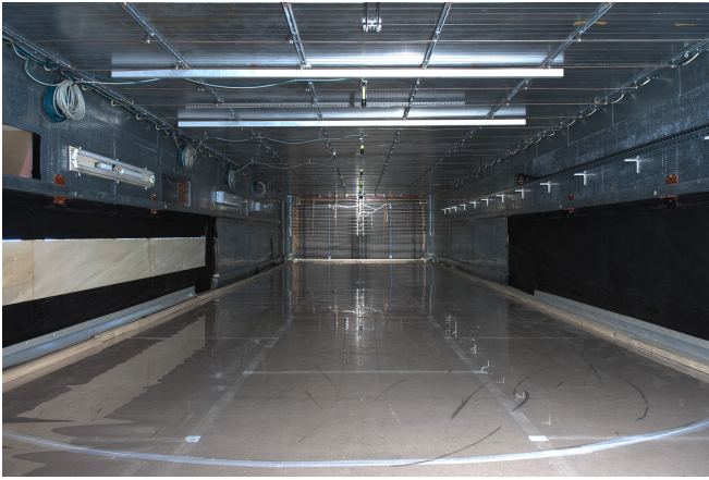
Fig. 2. The wind tunnel used for the experiments. The odor outlet hose is at the opposite end, centered on the floor.
