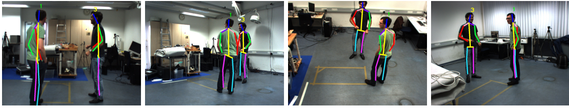
Figure 6.1 – Pose estimation results on the Shelf Dataset. The body poses are recovered in 3D and then projected onto the four camera views. The identity of each person, as indicated by the number on the top, is obtained by our tracker.
