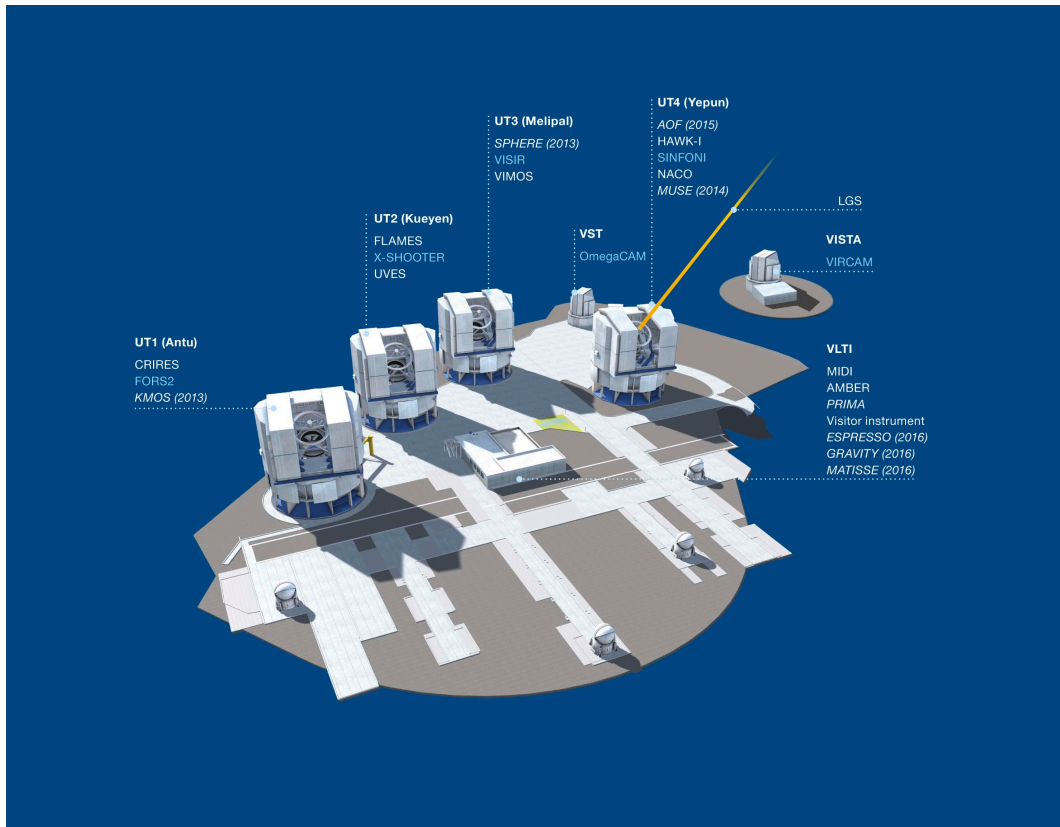
Figure 3.2: The map of the current instruments distribution among the four VLT Unit Telescopes. Source : http://www.eso.org/sci/facilities/paranal/instruments/overview.html
