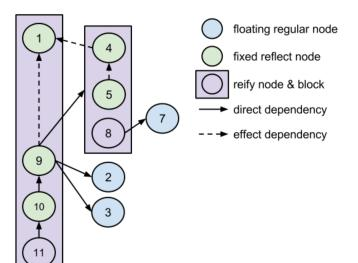
The schema illustrates how the Reify nodes fix the Reflect nodes in their block, whereas the scheduler can move pure nodes around. Now all nodes are reachable from the last statement (11) and thus the effectful statements will be scheduled and emitted too, as long as there are correct Reflect and Reify nodes to track all effects.
