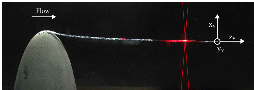
Figure 4.3: Photograph of the cavitating tip vortex and the LDV laser beams. The laser beams are crossing slightly underneath the vortex cavity center. W_\infty=10 m/s, \alpha=12^\circ , \sigma=1.7
