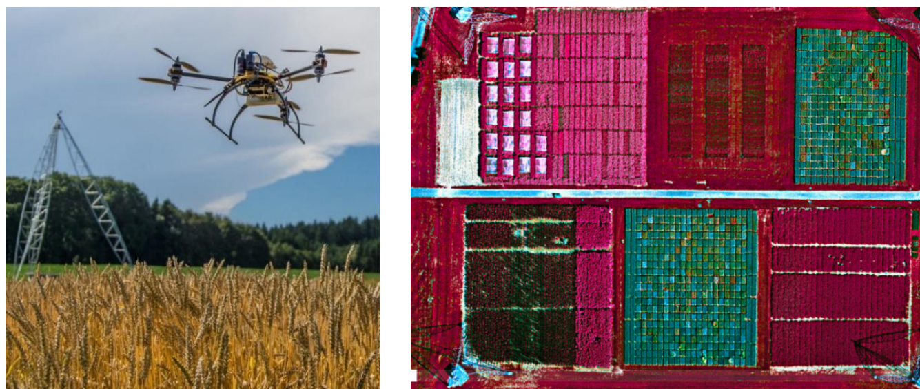
Figure 2. Airborne HSI platform based on a custom made hexacopter UAV (left) and the Principle Component Analysis (PCA)-based visualisation of the FIP area, which was used in the study (right).
