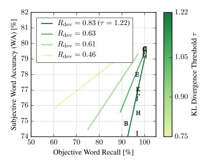
Figure 2: Relationship between word recall and word accuracy for different uncertainty thresholds  $\tau$  on a development set of 5 SUS recordings per TTS system. Lines indicate the linear fit at different values of  $\tau$  (for clarity, data points for the TTS systems "B" to "M" are shown for one threshold value only).
