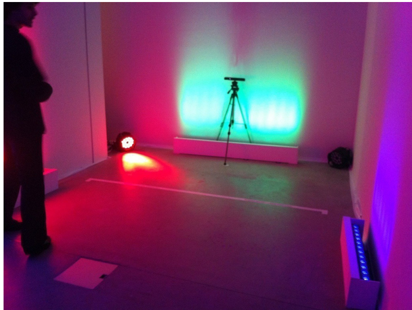
The single-user Aurora RGB mixer setup in the gallery space and in software representation. Each box represents a Teculmen lamp, the purple dot to the left is the tracked user. You can see how the blue lights on the right are dim, indicating the user is closer to the red.
