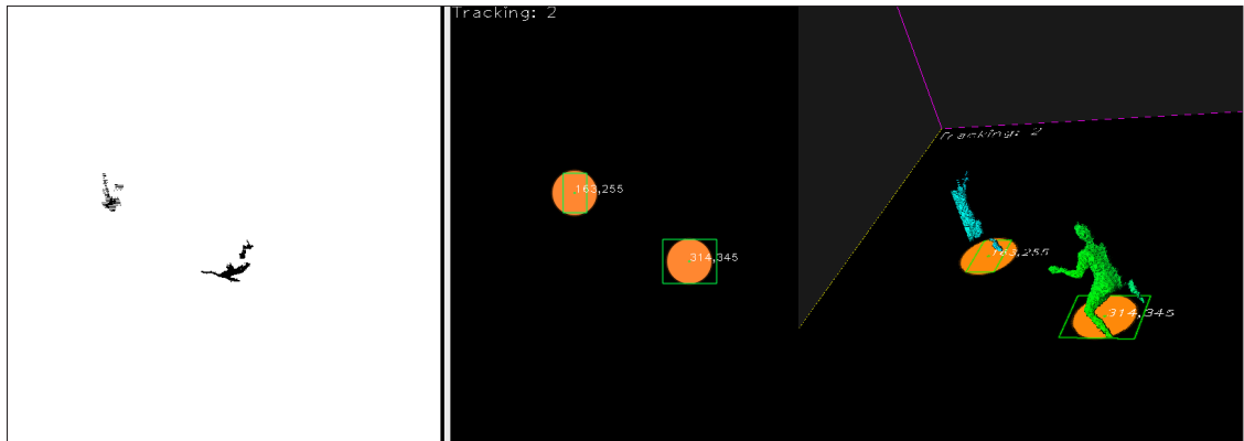
The three stages of “overhead” tracking using the point clouds. The far left shows the overhead view of the point cloud, adjusted to be high contrast. Running blob tracking on this results in the image in the middle, showing a centroid and bounding box. This can then be projected back onto the pointcloud data (third image).
