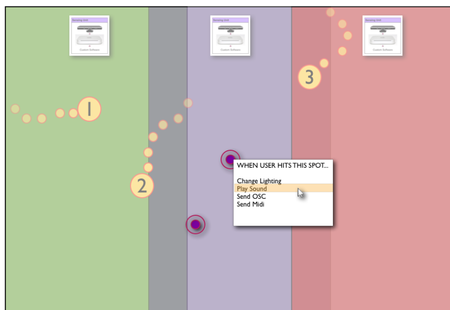
Conceptual sketches of the proposed system. Each colored rectangle represents the area covered by a single Kinect camera, the yellow dots represent users, the purple dots represent virtual “hotspots” which trigger events on stage.
