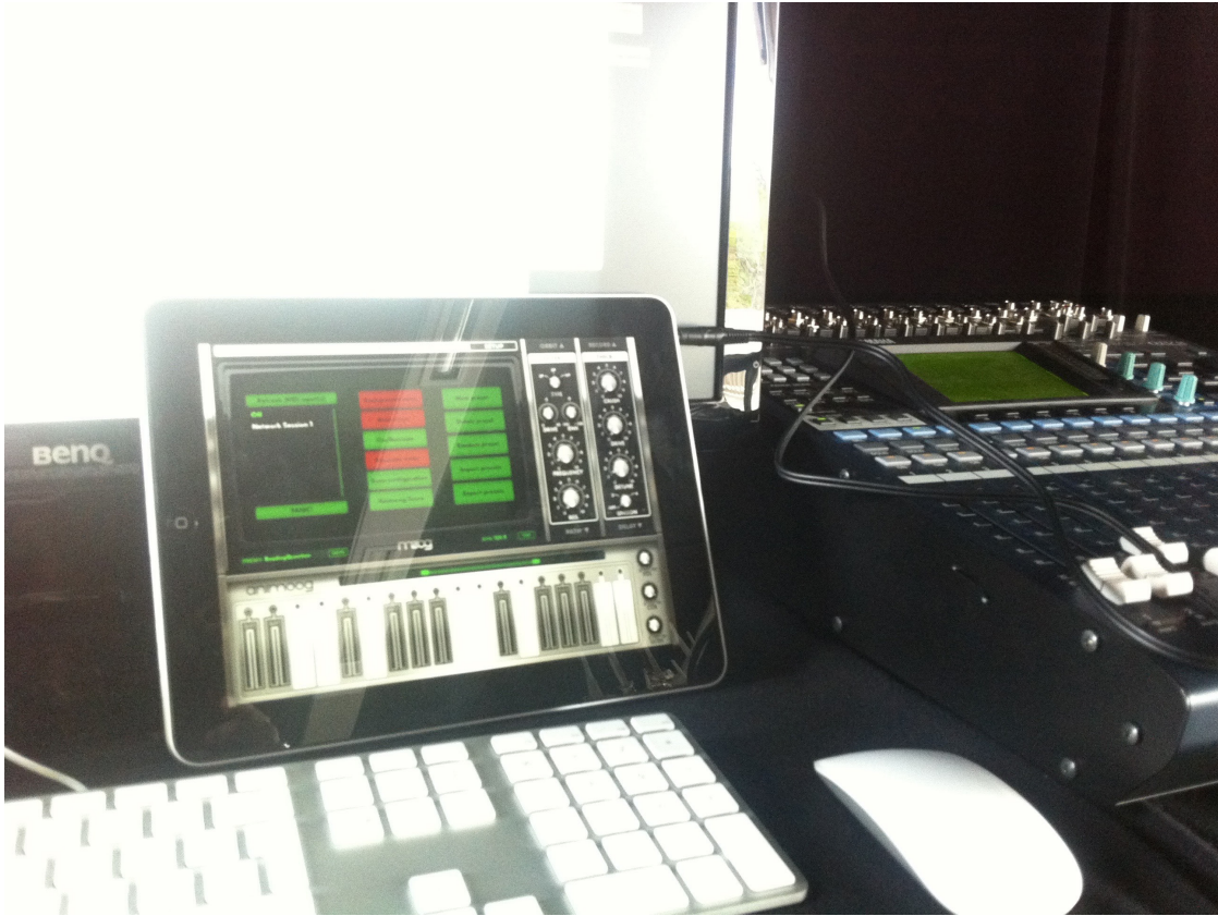
Prototype setup shows the NI-MATE output superimposed over a custom Processing sketch on the screen. The output is sent via wireless MIDI to the Animoog synthesizer running on the iPad, whose output is fed out through the PA system at the right.
