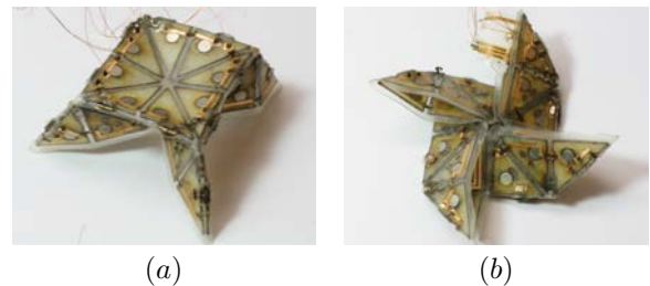
Fig. 6. Two programmed shapes of a robotic origami, table (a), and pinwheel (b).
