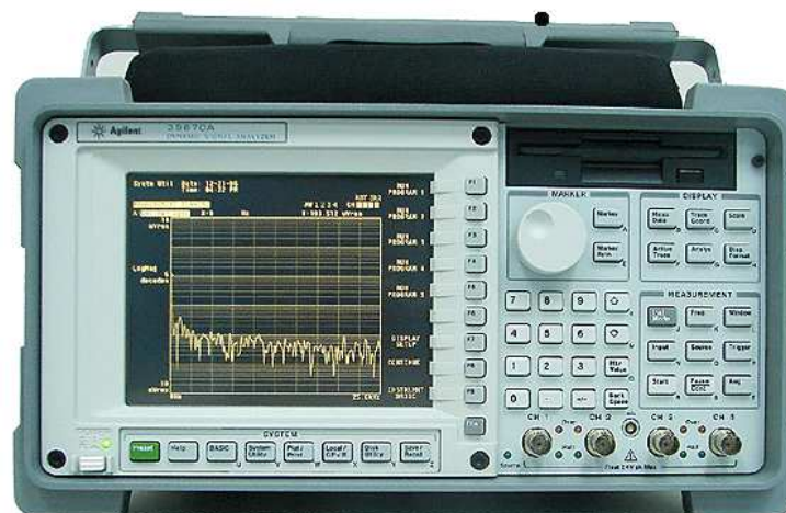
Figure 2.6 – Front view of the HP35670A Dynamic Signal Analyzer (photo courtesy of Hewlett-Packard©).
