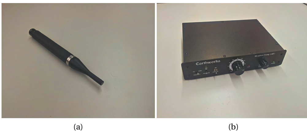
Figure 2.17 – Earthworks micro system: (a) M30BX microphone and (b) LAB1 preamp.
