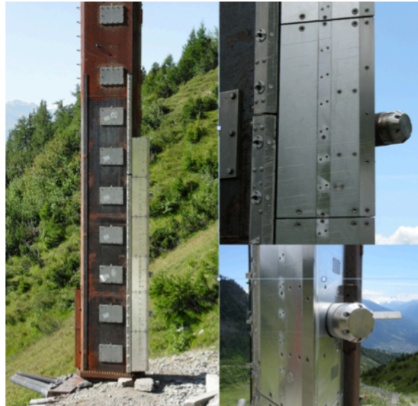
Fig. 1: The 20 m high tower is instrumented with high-frequency load cells, optical sensors for velocity measurements, capacitance probe for density measurements and flow depth sensors.
