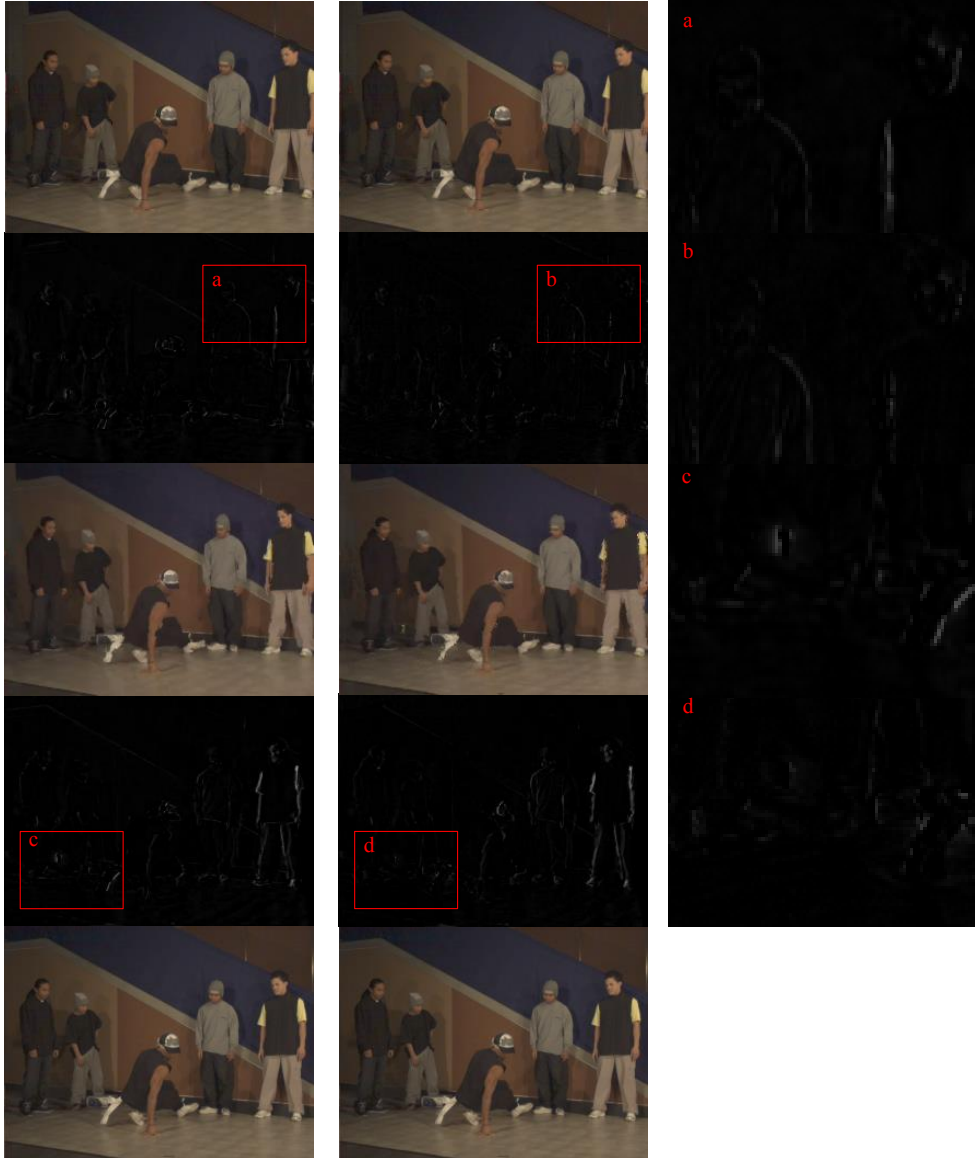
Fig. 9. Comparison of inter-view consistency for the Breakdancer sequence. Left: [13], Middle: proposed method, Right: Zoomed difference images. The first two columns show (from top to bottom): frame F_{v,t} , the difference of the warped frame from F_{v,t} to F_{v-,t} and frame F_{v-,t} , the reconstructed frame F_{v,t} , the difference of the warped frame from F_{v,t} to F_{v+,t} and frame F_{v+,t} , and frame F_{v+,t} , respectively. The third column shows the zoomed difference images from the first two rows. Errors were obtained by dropping one frame in V_1 . The zoomed parts of the difference images show higher inter-view consistency (smaller magnitude of the white color) of the proposed method compared to [13].
