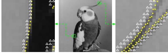
Fig. 4. Comparisons of the edge localization results with Canny edge detector [5] (white triangles) and the proposed annihilation-driven approach (yellow dots).
