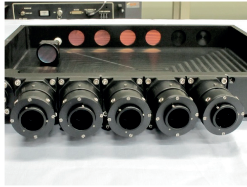
Fig. 2.1.6 Adjustable detector cells (with focusing optics) on front wall, four mirrors for beam cascading on rear wall
