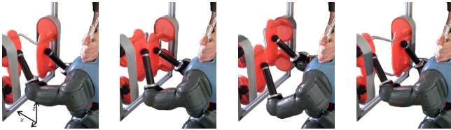
Fig. 5. Image sequence showing approximately one period of rotating the vertically mounted pedal racer with the arms of the COMAN robot after the learning, when the contact with the pedals is constantly kept. The attached video shows the complete experiment. The tape on the wheels simulates contact with the ground and keeps them at the same velocity, preventing the device from locking up, which happens if the front and the back wheels do not rotate together.
