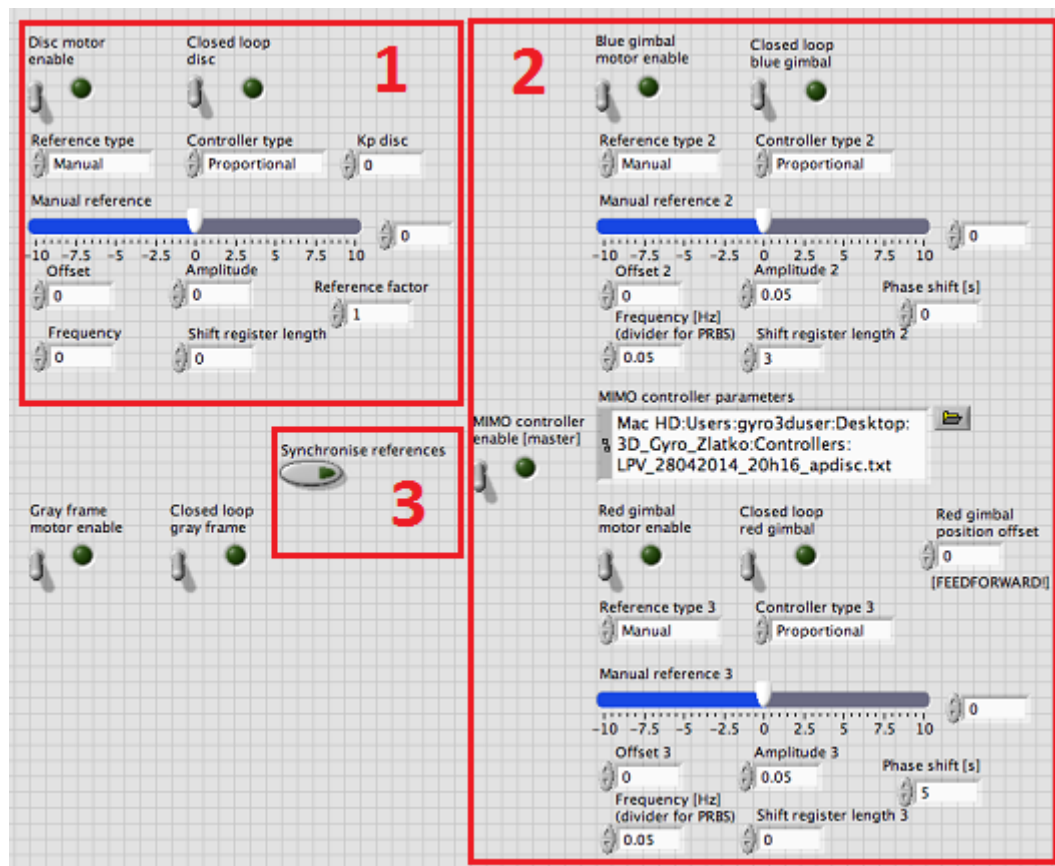
Figure A.3 – Several interface groups: 1) disk actuator group, 2) blue and red frame actuator group, 3) “synchronize references”
