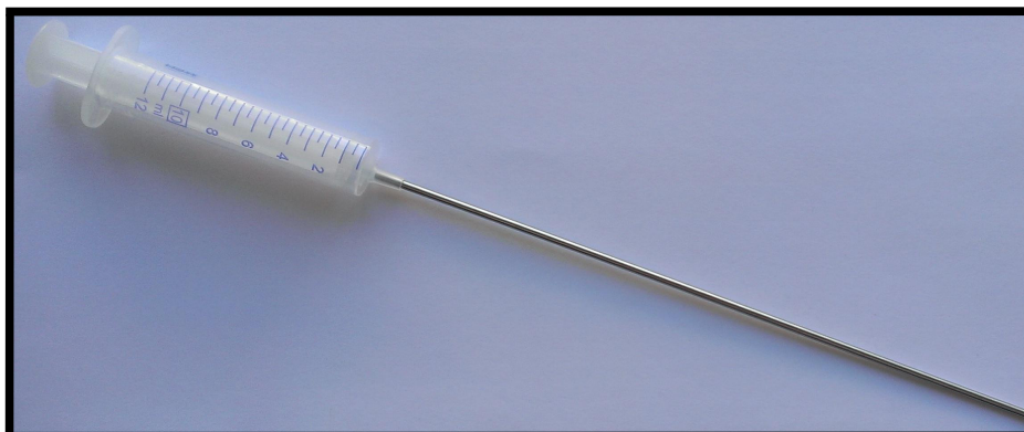
Figure A.1 – Home made syringe for inserting cement paste at the bottom of NMR tubes.
