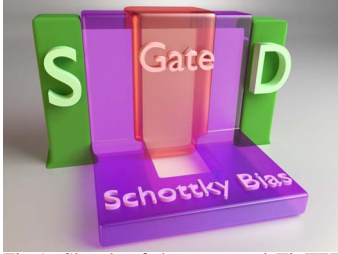
Fig.1. Sketch of the proposed FinFET. Violet: Schottky-Barrier Bias (SBB) region modulating the Schottky barriers. Red: Gate controlling the channel conduction.
