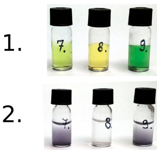
Figure 7. Photographs of shake-flask experiments after 24 h of the two-phase reaction. In row 1 the bottom phase is 5 mM DMFc in TFT solution. The upper phase in row 1 is flask 7: 0.1 M \text{HClO}_4 aq; flask 8: 0.1 M \text{NaClO}_4 aq; flask 9: 5 mM LiTB, 0.1 M \text{HClO}_4 . In row 2 are the aqueous phases (0.5 mL) taken from systems presented in row 1 after addition of 200 \mu\text{L} of 0.1 M KI and 10% starch.
