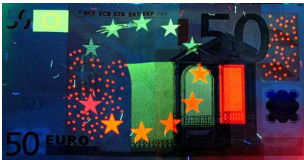
Figure S3. Fifty euro bank note shown under UV light and displaying luminescent parts (taken from Wikipedia)
