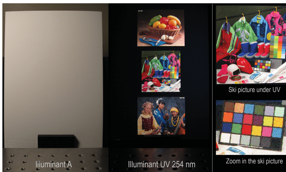
Figure 7. Photographs of a set of standard images reproduced with the luminescent inks on the Canson paper. On the left, a printed paper sheet under an A illuminant: the luminescent image is invisible. On the center, the same printed paper sheet under UV excitation at 254 nm: the luminescent images produced by the emission of the lanthanide complexes and of the blue emitting compound are visible and accurately reproduced. On the right, enlargements of the ski picture shown in the photograph on the center (i.e. viewed under UV light).
