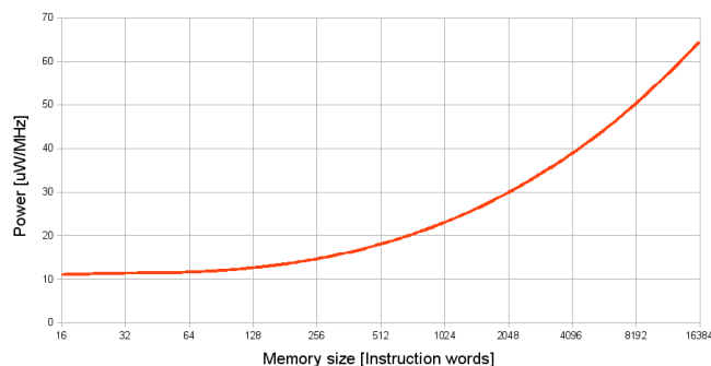
Fig. 1. Power consumption per access in 16-bit instruction word commercial 90nm SRAMs.
