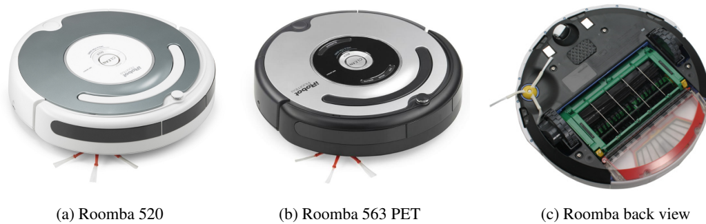
Figure 3.2: Two different models of the Roomba were used in this study. Households without a pet received model (a), those with a pet received model (b) which is specifically adapted to vacuum pet hair, additionally has a time scheduling function, and comes with two so-called “virtual walls” (infrared barrier) that help keeping the robot in a specific area.
