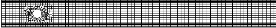
Fig. 2. Scheme of the generated mesh in the domain (the real mesh is 8 times finer than this one).
