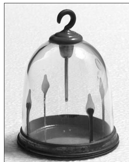
Figs. 2 Paul – de Saussure electroscope. Base diam. 70 mm; height 70 mm.
