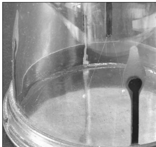
Fig. 4 Close-up of the pith balls suspended by thin metal wires.
