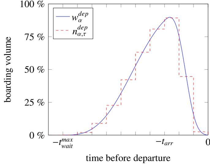
Figure 2: Illustration of the accumulation of outbound passengers on a platform prior to train departure (adapted from Tolujew and Alcalá, 2004). The earliest passengers arrive at a time  $t_{wait}^{max}$  before departure, and boarding starts shortly after the arrival of the train at  $t_{arr}$ , causing a drain of passengers.
