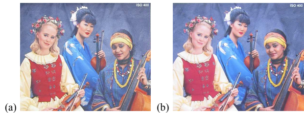
Figure 10. (a) Picture of orchestra print on the metal film viewed under specular reflection, taken with an exposure of 1/320 s and (b) picture of orchestra print on paper, taken with an exposure of 1/125 s, under the same illumination and capturing geometry (for details: see the electronic version).
