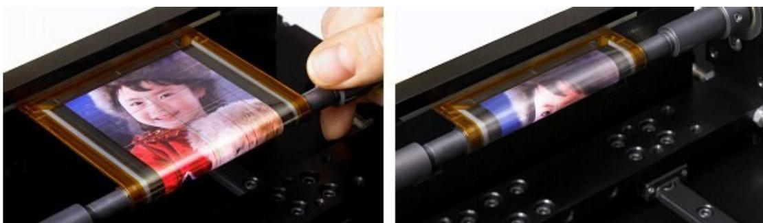
Figure 4: Rollable OLED display driven by OTFT by Sony.
