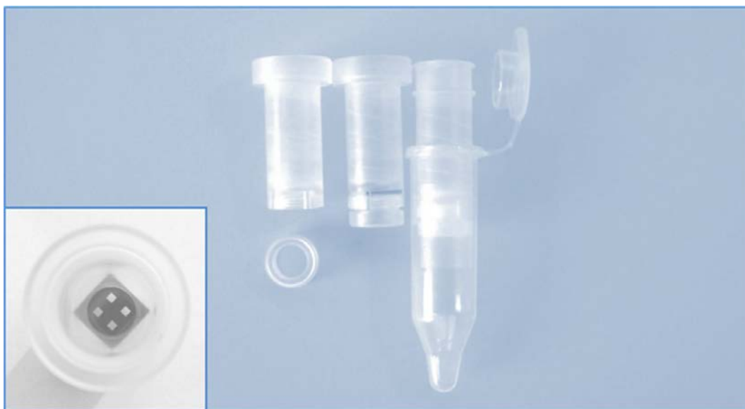
Figure A.1.1 Standard commercially available 2 mL centrifugal tube in which a specifically designed tube integrating NSiMs and the solution of interest can be sled in.
