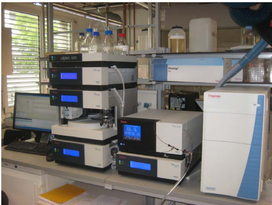
Fig. (4B). Checking the chemical integrity of chemical compounds using an UHPLC-MS system. To estimate the purity of the whole collection within a reasonable time frame, an ultra high performance liquid chromatography system connected to different detectors (Mass spectrometer, UV and CAD) was installed and the workflow from data acquisition to data processing has been validated. Hits from screens will be systematically analyzed and it is planned to randomly analyze the whole ACCESS collections according to the throughput.
