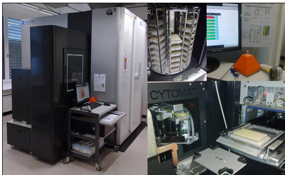
Fig. (4A). Compound management using an automated storage system. Compounds dissolved at a concentration of 10 mM in dimethyl sulfoxide in 2D-bar coded capped tubes (300 \mu L) are stored at -20^{\circ}\text{C} in an automated store in a controlled low humidity environment. Plated compounds are also stored in the system using sealed 1D coded 384 well plates. Compound tracking and inventory is performed by a Laboratory Information Management System (LIMS) developed by the BSF.
