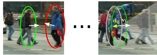
Fig. 4. Role of the visual motion for tracking. Left: Detection r_i at time t_i along with its estimated visual motion \mathbf{v}_i (green ellipse). Right: in subsequent frames, the motion cost associated to this detection favors associations with other detections located in the direction of motion (shaded area) and penalizes associations in opposite directions (example of blue person, gray ellipse).
