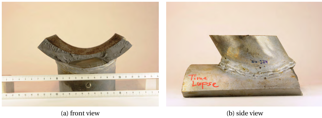
Figure 5.28: Cracking of joint S10-J3N (tensioned brace side).
