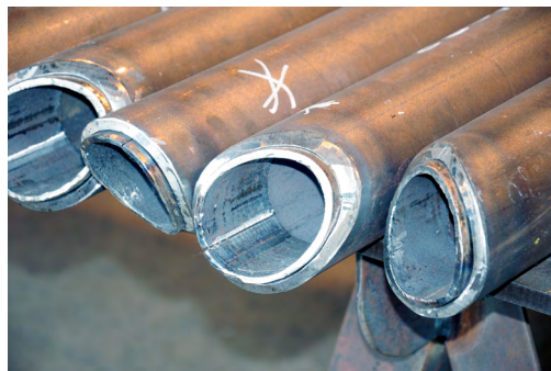
(a) Beveled brace ends with backing rings.
