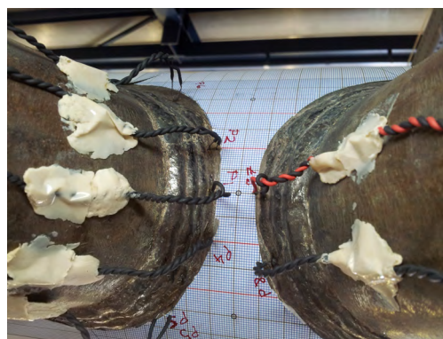
(b) Twisted wire probes attached to the cracking sites.
