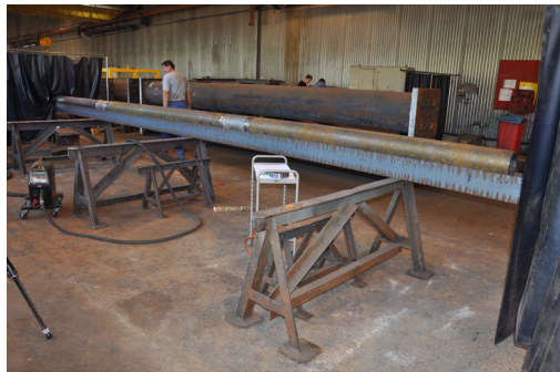
(a) Tack-welding of cast joints on a straight platform.
