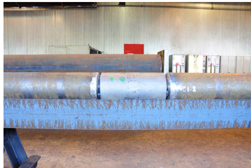
(b) Cast joint and tubes fitted-up.
