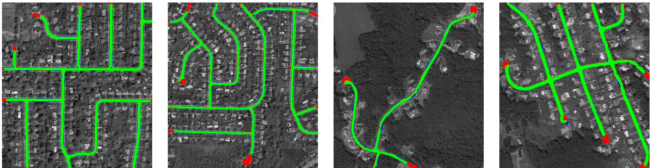
Figure 9. Qualitative results on road tracking. Gree is true positive, blue false positive, red false negative.
