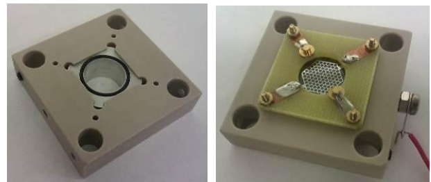
Figure 3. Simple BB holder, with and without thruster chip present.
