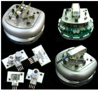
Fig. 4. Khepera III and KheNose with sensing modules
