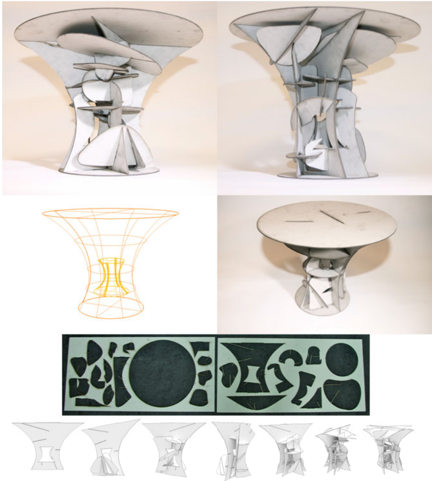
Fig. 1 A physical table built with orthogonally intersecting planar pieces using our design method. Also pictured are the hull wireframe, the negatives of the corresponding pieces, and the building process.
