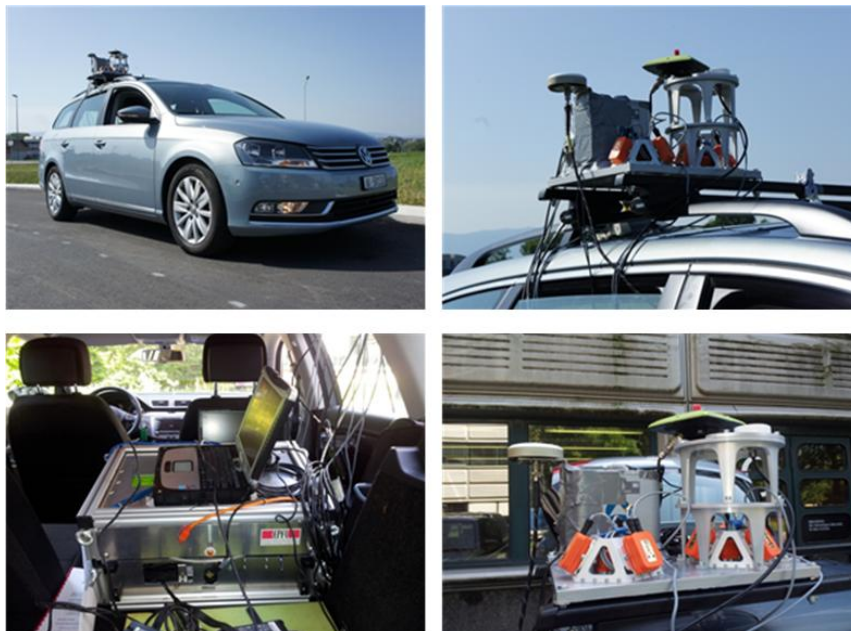
Figure 25. Measurement platform mounted on the test vehicle.
