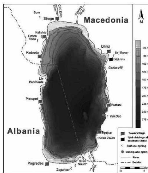
Figure 1: Map of Lake Ohrid. Bathymetry with 25 m contour intervals and marked surface and subaquatic sources (Albrecht, 2008)
